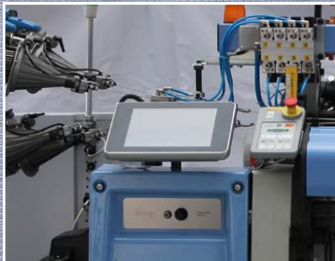
Automatic Setting of the Relay Nozzle Pressure
